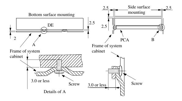
Figure 3.2 Mounting frame structure
